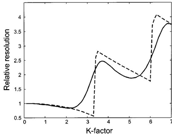
Fig. 5. Resolution improvement of the output signal as a function of reference pulse power  $K$ . Dashed curve, FWHM criteria; solid curve, standard deviation measure.
