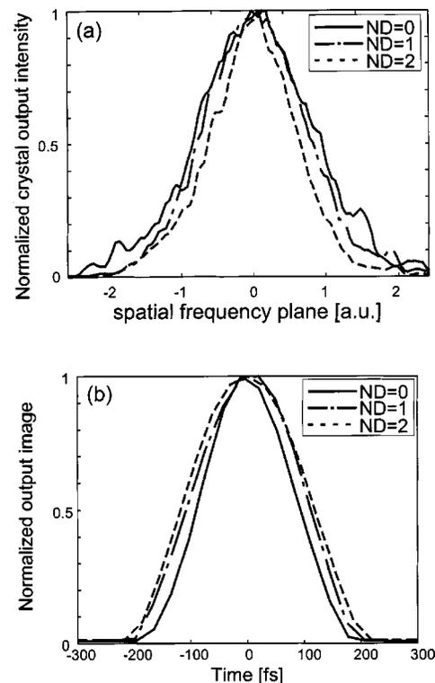
Fig. 7. Experimental results: (a) intensity distribution in the Fourier plane, (b) output pulse image, as functions of the reference pulse attenuation. A high ND setting corresponds to a small  $K$  value. Broadening in the Fourier plane and narrowing in the corresponding pulse images are exhibited.
