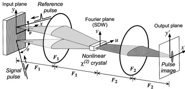
Fig. 1. Time-to-space conversion by using wave mixing of inverted spectrally decomposed waves from a signal and a reference pulse:  $F_1$ ,  $F_2$ , focal length.
