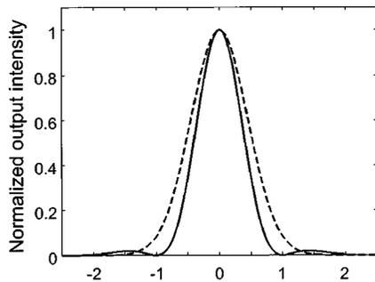
Fig. 4. Enhanced-resolution imaging: comparison of the output image for linear (dashed curve) and nonlinear (solid curve for  $K = 2.5$ ) conversions.
