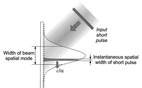
Fig. 2. Gaussian beam mode and Gaussian pulse envelope incident on the diffraction grating. The ratio of their spatial widths determines the resolution of the system.
