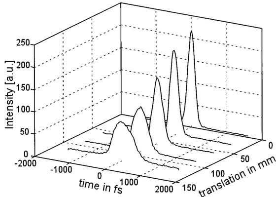
Fig. 3. Synthesized temporal waveforms generated by a quadratic wave front in the spatial channel, generating chirped pulses. The quadratic wave front is generated by longitudinal translation of a point source from the input plane.
