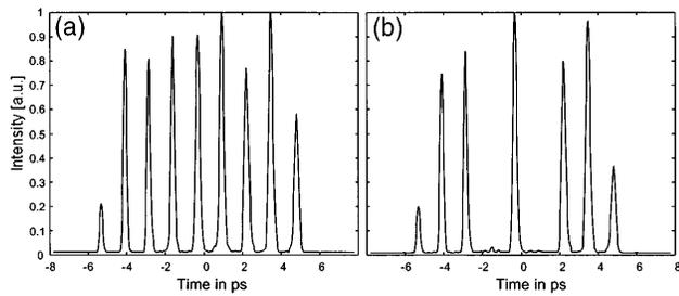
Fig. 2. Synthesized temporal waveform generated by a spatial-information mask consisting of a sequence of equally spaced point sources. (a) All points are illuminated by quasi-monochromatic light. (b) Two point sources are blocked.
