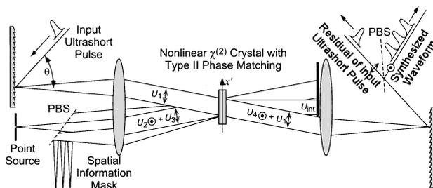
Fig. 1. Experimental setup of the spatial-temporal processor: The CSN results in information exchange in a four-wave-mixing process equivalent. PBS's, polarizing beam splitters.
