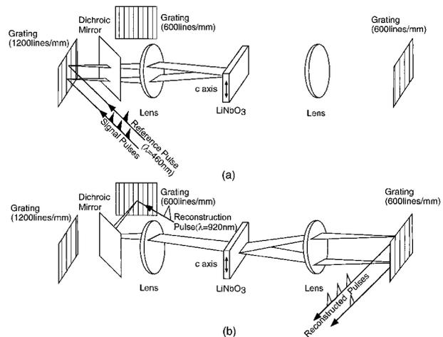
Fig. 1. Time-domain storage system using a spectral holographic recording system: (a) recording setup, (b) reconstruction setup.
