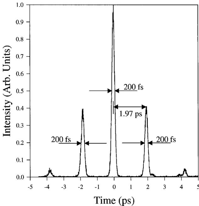
Fig. 2. Trace from an autocorrelator showing the reconstructed time sequence stored in a spectral hologram.
