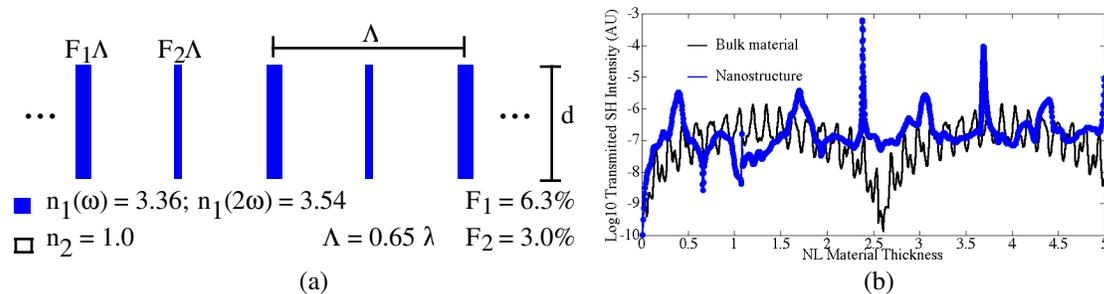
Fig. 1. (a) Schematic of enhanced SHG nanostructure having two differing grooves per grating period; (b) Transmitted second harmonic output (Log10 scale) versus nonlinear material depth for a bulk material and the nanostructure.
