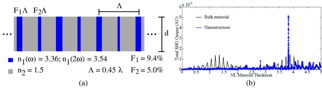
Fig. 2. (a) Enhanced-SHG nanostructure composed of GaAs and oxidized AlAs; (b) Transmitted second harmonic intensity versus nonlinear material depth for a bulk material and the nanostructure.
