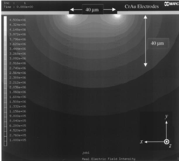
Fig. 4. Two-dimensional cross section of the electric-field strength distribution within PLZT for a surface-electrode device with electrodes separated by 40  $\mu\text{m}$  and a potential difference of 124 V. Charge buildup at the corners of the electrodes results in a large gradient of the electric field within the electrode gap near the surface of the device.
