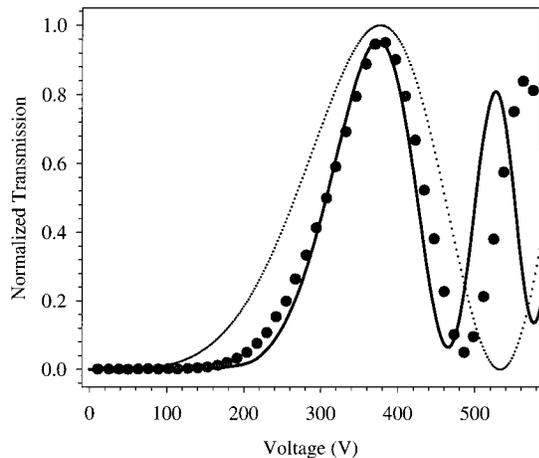
Fig. 6. Simulation (solid curve) of the surface-electrode device performance, with an electrode gap of  $500\ \mu\text{m}$  for PLZT 9.0/65/35 that is  $388\ \mu\text{m}$  thick, and experimental data for a fabricated device (circles) in comparison with the simulation results (dotted curve) with the commonly employed Jones calculus and quadratic EO model.
