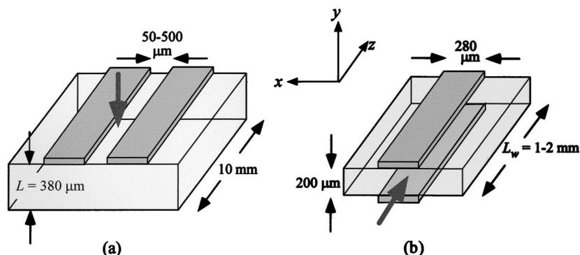
Fig. 3. (a) Surface-electrode device in which CrAu electrodes are evaporated onto the surface of the PLZT wafer and light is normally incident on the surface (along the  $y$  axis). (b) Transverse-electrode device in which electrodes are on opposite sides of the wafer and light is normally incident on the polished edges (along the  $z$  axis).
