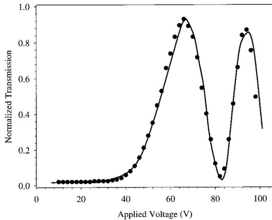
Fig. 8. Experimental data (circles) and simulated results (curve) of transmission through the central  $20\ \mu\text{m} \times 20\ \mu\text{m}$  area of the transverse-electrode device with  $280\text{-}\mu\text{m}$  electrodes separated by  $200\ \mu\text{m}$  of PLZT 9.0/65/35 [see Figs. 7(a) and 7(b)].
