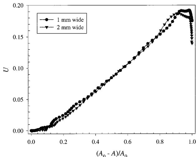
Fig. 2. Depolarized light (normalized) intensity as a function of the polarized-light intensity for identical PLZT samples with propagation lengths of 1 and 2 mm.
