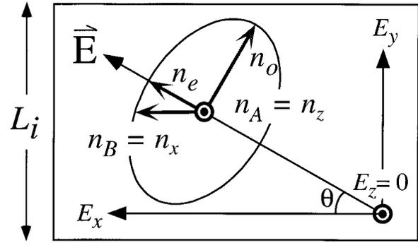
Fig. 5. Single element of the 2-D cross section where we calculate an average electric-field magnitude and direction. We show the variation of the index ellipsoid following the direction of the electric field.
