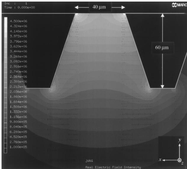
Fig. 1. FEA-calculated electric-field strength distribution for trapezoid-shaped embedded electrodes separated by 40 and 60  $\mu\text{m}$ , with a potential difference of 124 V.
