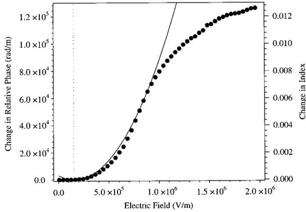
Fig. 5. Change in the relative phase calculated from measured data for PLZT 8.9/65/35 (circles). For comparison we also show the calculated change in phase obtained by use of a shifted ( $E_0 = 1.5 \times 10^5$  V/m) electric field in the standard quadratic model (solid curve) with the quadratic EO coefficient  $R = 17.0 \times 10^{-16}$  (m/V)<sup>2</sup>. The change in the index of refraction is calculated by use of the linear relation  $\Delta\phi/L = 2\pi\Delta n/\lambda$ .
