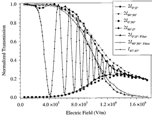
Fig. 4. Seven optical intensity measurements normalized to illustrate the envelope functionality of the vertical and horizontal components to the  $I_{45^{\circ},45^{\circ}}$  data.
