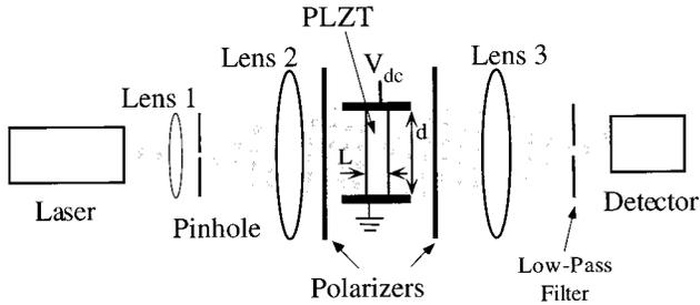
Fig. 2. Experimental setup for the characterization and modeling of PLZT samples. The PLZT sample is fully illuminated to avoid localized photorefractive effects. The low-pass filter was only used for experimental measurements for which the scattered fields needed to be filtered out.
