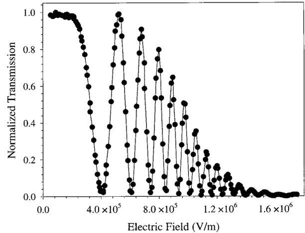
Fig. 3. Using a low-pass filter (see Fig. 2), we remove the scattered light from the detected signal. The remaining dc component contains no optical bias, allowing us to conclude that the dc light is polarized. In this measurement we used parallel polarizers, which resulted in a maximum intensity at zero voltage. The PLZT sample used was 1 mm thick, which accounts for the increase in phase variation compared with Fig. 1(b).
