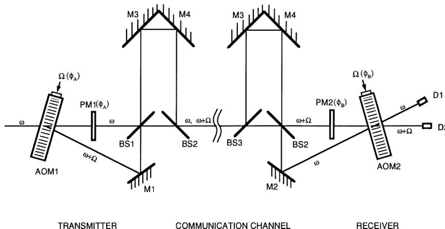
Fig. 2. Schematic diagram of the lossless frequency-division long-distance interferometer. M's, mirrors.
