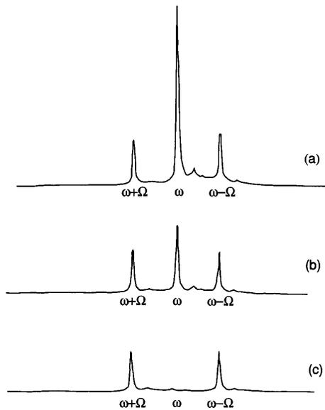
Fig. 3. Experimental results recorded at the output 1 of Fig. 1 by a scanning Fabry-Perot interferometer integrated with a photodetector: (a)  $\phi_A - \phi_B = 0$ , (b)  $\phi_A - \phi_B = 2\pi/3$ , (c)  $\phi_A - \phi_B = \pi$ .
