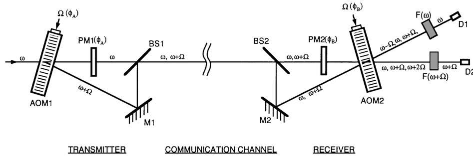
Fig. 1. Schematic diagram of the frequency-division long-distance interferometer. M's, mirrors.
