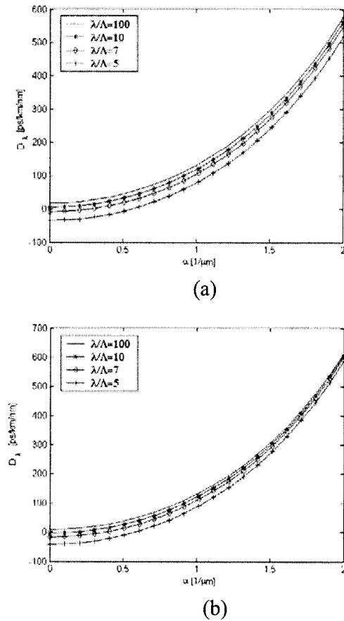
Fig. 6. Total linear dispersion coefficient versus angular frequency  $\alpha$  in a fused-silica-air periodic structure (fill factor  $f = 0.5$ ): (a) TE polarization and (b) TM polarization.
