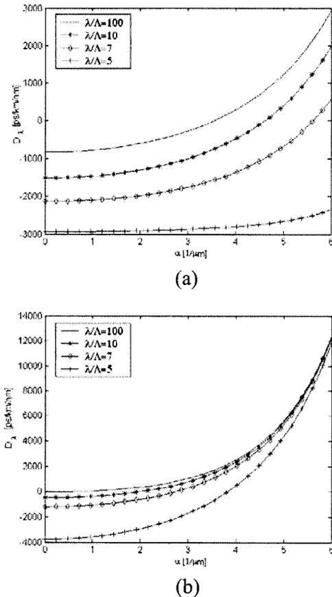
Fig. 5. Total linear dispersion coefficient versus angular frequency  $\alpha$  in a GaAs-air periodic structure (fill factor  $f = 0.5$ ): (a) TE polarization and (b) TM polarization.
