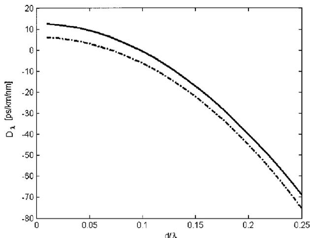
Fig. 4. Total linear dispersion coefficient versus  $d/\lambda$  in a fused-silica-air periodic structure (fill factor  $f = 0.5$ ) for TE (solid curve) and TM (dashed-dotted curve) polarization states.
