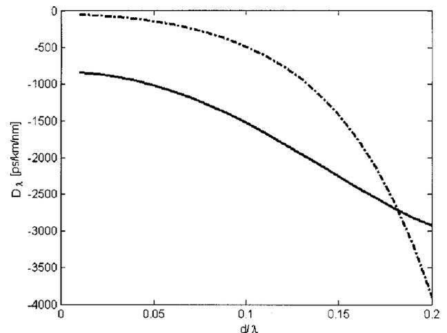
Fig. 3. Total linear dispersion coefficient versus  $d/\lambda$  in a GaAs–air periodic structure (fill factor  $f = 0.5$ ) for TE (solid curve) and TM (dashed-dotted curve) polarization states.
