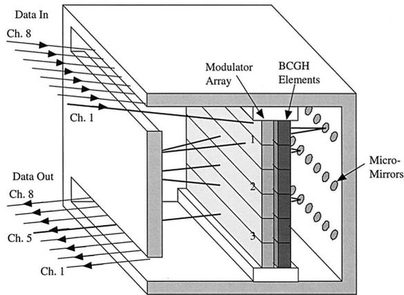
Fig. 5. Folded  $8 \times 8$  optical MIN with one input beam, shown propagating from channel 1 to channel 5. In this example there are three stages of DBS's, which require three round-trip travels in the micromirror cavity.
