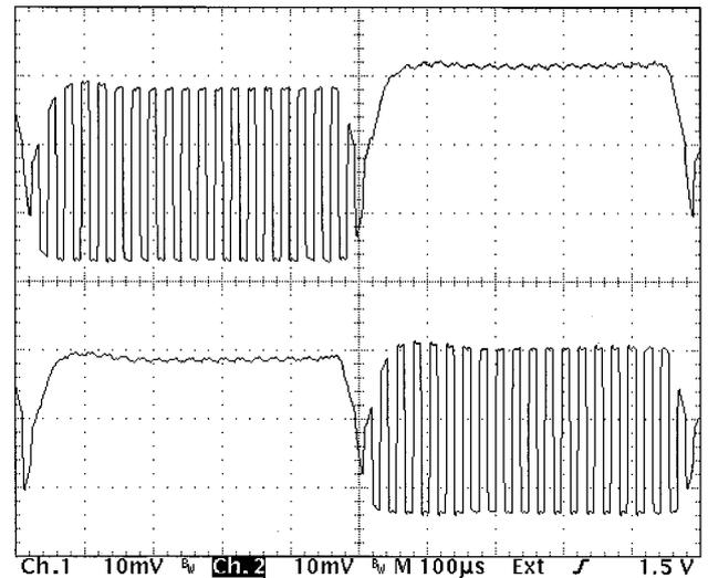
Fig. 9. Output signals for a single folded DBS ( $2 \times 2$  switch) with two input signals: a dc signal and a 20-kHz signal. The switch is reconfiguring at a 1-kHz rate, limited by the 100- $\mu\text{s}$  characteristic rise time of the FLC. The measured average SNR is 57:1.
