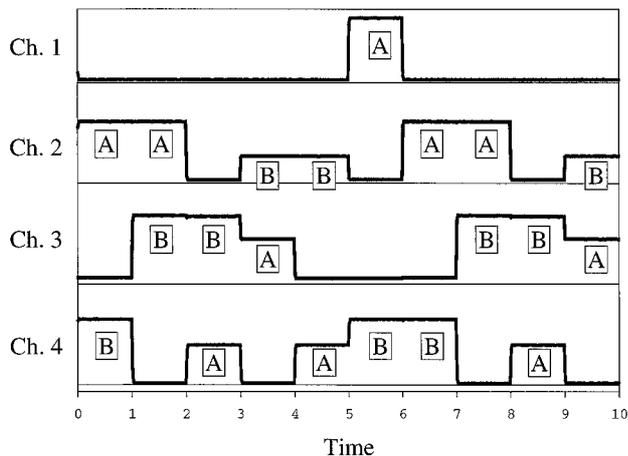
Fig. 10. Output from a  $4 \times 4$  switch with two input signals (A and B) routed to the four output channels by a host computer controller. The average SNR is 120:1, which is twice as great as that of the single DBS performance, highlighting the filtering capabilities of the folded MIN configuration.
