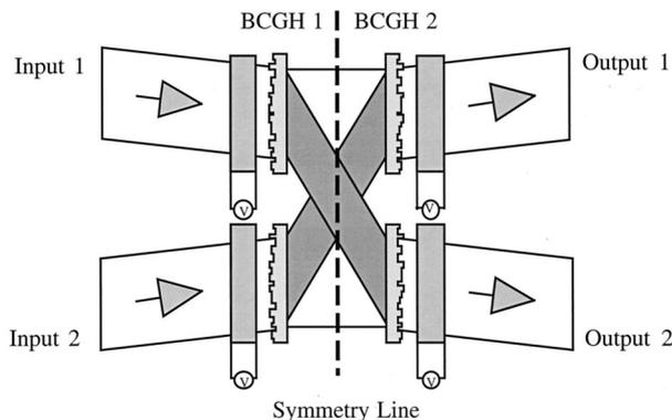
Fig. 3. Optical implementation of the DBS. Each BCGH element performs  $1 \times 2$  switching, depending on the state of the polarization-rotator element. The input and the output states of the two channels are identical, permitting filtering with a polarizer of linear cross talk at the output.
