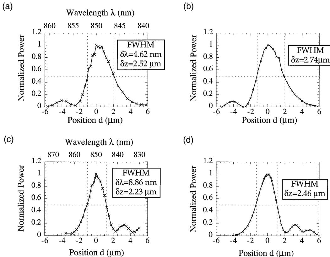
Fig. 3. Experimental results of the longitudinal PSF: chromatic confocal microscope with the (a) 40 $\times$  objective, (c) 60 $\times$  objective and the conventional confocal microscope operating at the design wavelength  $\lambda_d = 850$  nm with the (b) 40 $\times$  objective, (d) 60 $\times$  objective.
