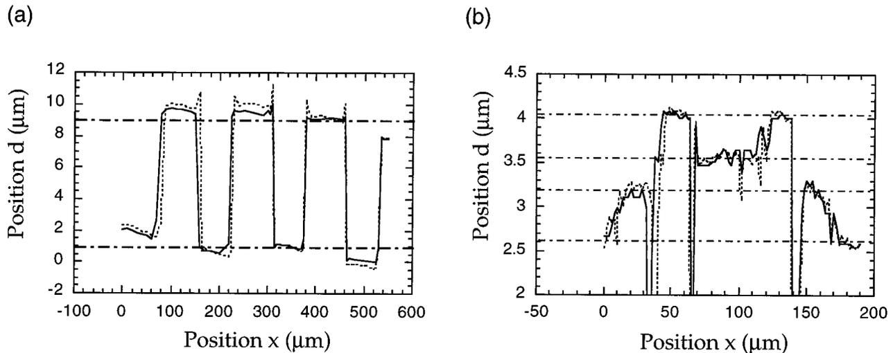
Fig. 4. Experimental results of measuring surface-relief profiles with the conventional (solid curves) and chromatic (dashed curves) confocal microscopes: (a) binary grating profile, (b) four-phase-level DOE. (The horizontal lines highlight the sample level positions.)
