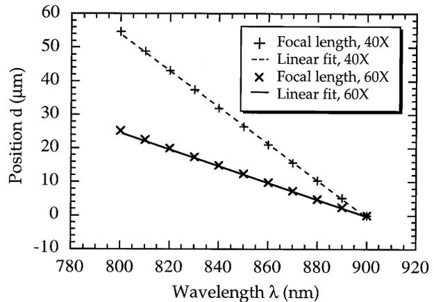
Fig. 2. Experimental results of system characterization: wavelength-to-depth mapping.
