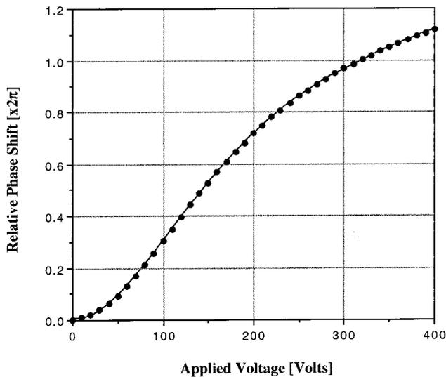
Fig. 8. Average measured phase-modulation response of the PLZT modulators in the 32-channel phased-array device shown in Fig. 7.
