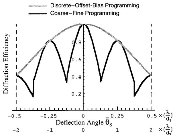
**Fig. 12.** Comparison of the DE versus the scan angle of an aligned two-stage phased-array deflector cascade by use of the discrete-offset-bias protocol (upper curve) and the coarse-fine protocol (lower curve). Cascade configuration:  $M_1 = 4$ ,  $M_2 = 8$ , 100% filled apertures; minimum control-line arrangement (Fig. 4).
