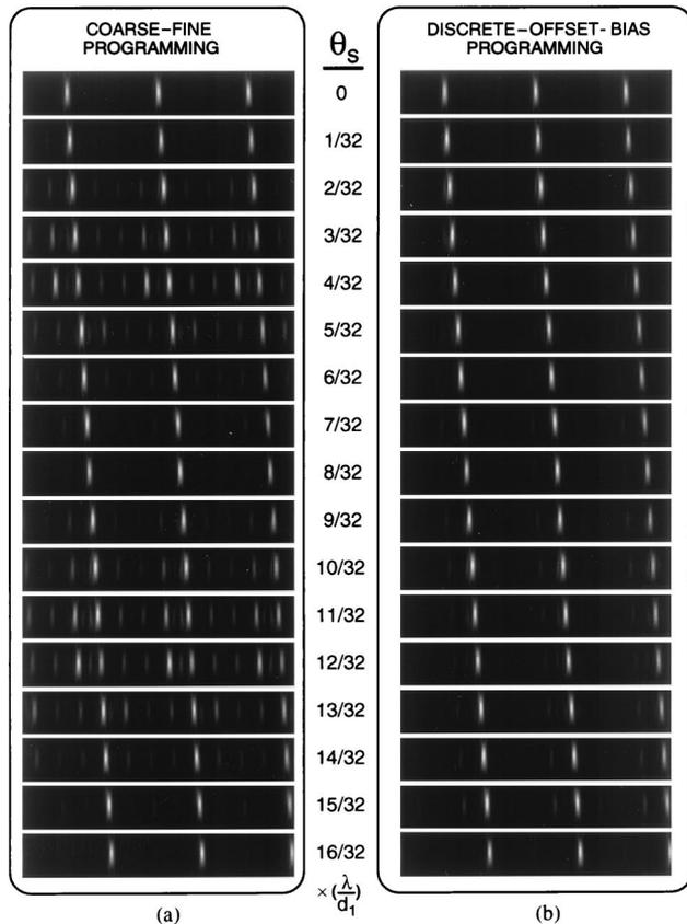
Fig. 9. One-dimensional beam-steering output by use of two 32-channel PLZT phased arrays in an aligned two-stage cascade with  $M_1 = 4$  and  $M_2 = 8$ . The cascaded arrays were programmed for deflection to various angles  $\theta_S$  by use of (a) the coarse-fine protocol and (b) the discrete-offset-bias protocol. Only half of the 32 resolvable scan outputs are shown.
