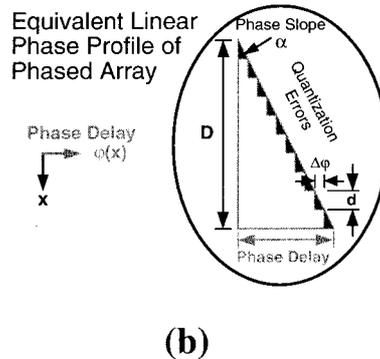
Fig. 1. Basic concept of a 1-D phased-array deflector: (a) near-field layout and far-field intensity pattern, and (b) equivalent phase profile of the 1-D array (with unfolded phases). Quantization errors are shown as dark notches.
