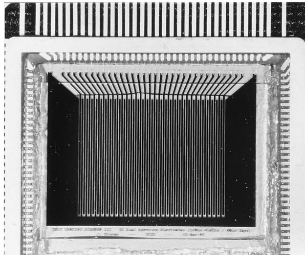
Fig. 7. Packaged 32-channel optical phased array made with PLZT. The active window has dimensions of 12.8 mm  $\times$  10.0 mm.
