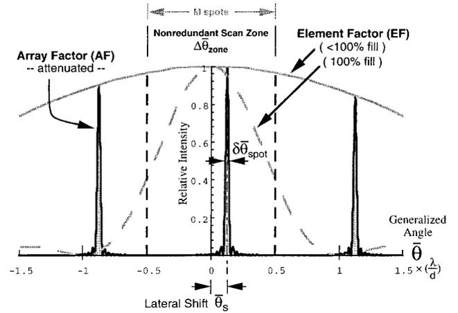
Fig. 2. Central lobes of the normalized far-field intensity pattern  $I^{\text{OUT}}(\bar{\theta})$  of a 1-D echelon grating deflector with  $M = 32$  channels, a fill factor of  $w/d = 1/5$  [solid envelope curve (EF)], and a deflection angle of  $\bar{\theta}_S = (1/8)(\lambda/d)$ . The ideal fill-factor envelope ( $w/d = 1$ ) is shown as a dashed curve.
