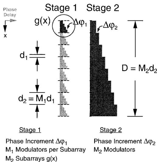
**Fig. 4.** Schematic layout of the unfolded phase distribution of an aligned two-stage phased-array cascade with a minimum control-line configuration.
