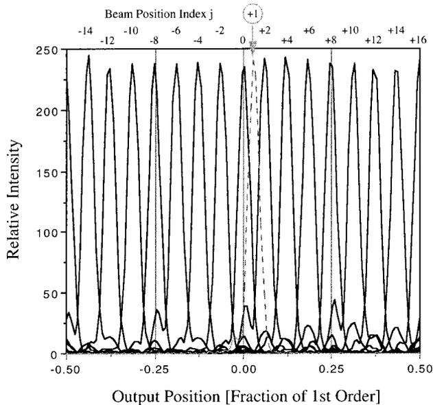
Fig. 11. Intensity profiles of the two-stage deflector output for the primary deflection angles of  $\theta_S = j/32(\lambda/d_1)$ ,  $j = -14, \dots, +16$  (solid curves) and  $j = +1$  (dashed curve) under discrete–offset-bias programming. The data cover the central nonredundant scan zone in the output.
