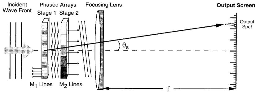
Fig. 3. Basic optical layout of a two-stage phased-array cascade with a reduced number of external connections. Stage 1 is addressed by  $M_1$  control lines and stage 2 by  $M_2$  control lines. By itself, stage 1 can deflect to only discrete output angles (shown as thick tick marks on the output screen).
