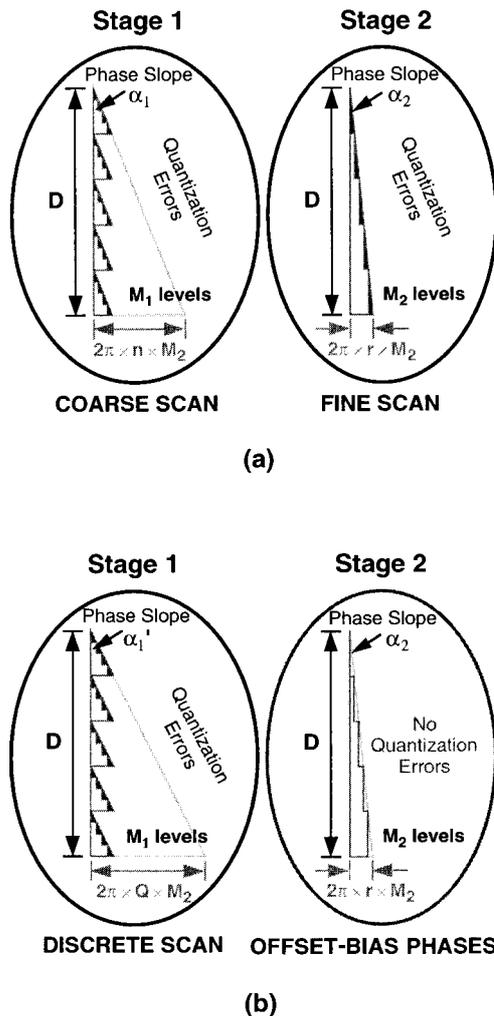
Fig. 5. Two basic strategies for programming an aligned two-stage phased-array deflector of the form given in Fig. 4. Equivalent phase profiles for the two stages are shown: (a) Coarse-fine programming; quantization errors occur in both stages. (b) Discrete-offset-bias programming; only stage 1 exhibits quantization errors.
