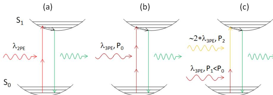
**Fig. 1.** Schematic energy diagram demonstrating degenerate and non-degenerate multi-photon excitation of a molecule: (a) degenerate 2-photon excitation; (b) degenerate 3-photon excitation; and (c) non-degenerate 2-photon excitation.
