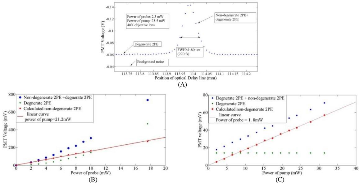
Fig. 3 (a). The beam profile of the fluorescence obtained by scanning the time delay line. (b). Power dependence of the fluorescence with varied power of probe beam and fixed power of pump beam. (c) Power dependence of the fluorescence with varied power of pump beam and fixed power of probe beam.
