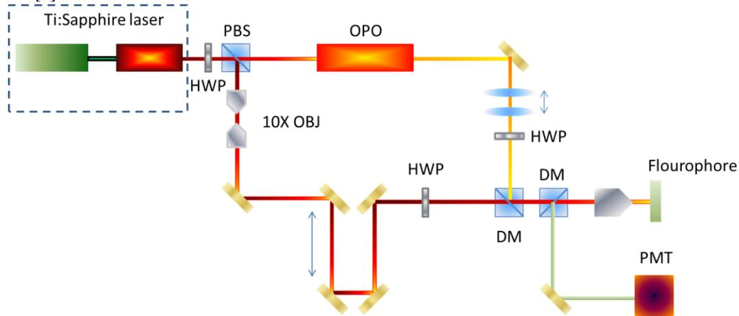
**Fig. 2.** Experimental setup for non-degenerate 2-photon excitation. PBS-polarizing beam splitter; OPO-optical parametric oscillator; OBJ-objective lens; HWP-half wave plate; PMT- photomultiplier tube.
