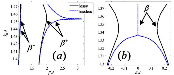
Fig. 2. (Color online) (a) Dispersion relations of the  $\beta^+$  and  $\beta^-$  modes for chains of lossless and lossy gold ellipsoids with spacing  $d = 72$  nm, twist angle  $\phi_0 = 18^\circ$ , and major and minor axes of lengths of 34 and 17 nm, respectively. (b) Dispersion relations of the  $\beta^-$  mode for the same chain but with twist angle  $\phi_0 = 85^\circ$ .
