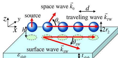
Fig. 1. (Color online) TWs on an array of nanoshells above a surface can radiate into SWs and space waves.
