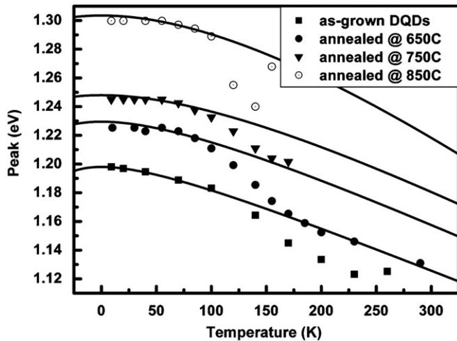
Fig. 4. The temperature-dependence curves of the PL peak energies of as-grown DQDs and samples at different annealing temperatures. The solid lines are fitted by the Varshni equation.
