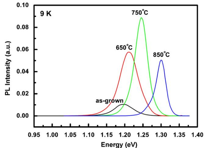
Fig. 3. PL spectra at 9 K of as-grown DQDs and samples annealed at different temperatures of 650, 750 and 850 °C for 30 s.
