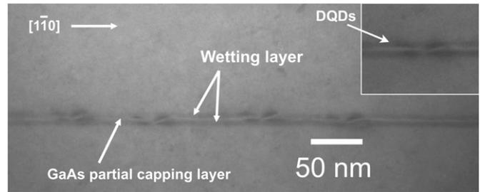
Fig. 2. Cross-sectional TEM image of DQDs using partial-capping-and-regrowth process.
