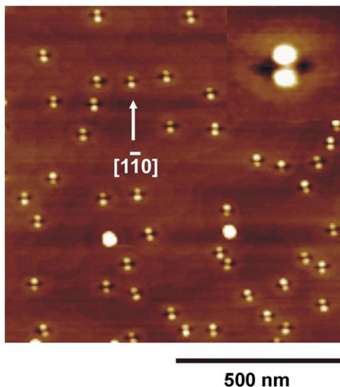
Fig. 1. AFM image of as-grown DQDs. The inset is high-contrast image.
