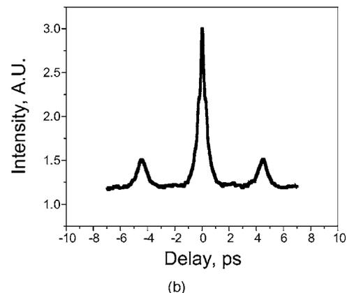
Fig. 4. Experimental intensity ACTs of signals with 7 GHz modulation. RF power is maintained at 15 dBm while the bias voltage is varied. (a) ACT in the presence of a strong dc component in the modulating signal  $\nu(t)$ . Experimental result shows agreement with the trace obtained from our linear model in Fig. 2(b). (b) ACT when the modulator was null biased. The autocorrelation process leads to the formation of three pulses as the inner two satellite pulses drop out.
