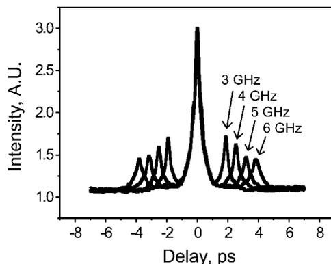
Fig. 5. Overlaid experimental intensity autocorrelations showing the effect of increased modulation frequency on a pulse-shaped waveform. The temporal broadening of the 6 GHz upshifted and downshifted pulses is apparent when comparing its FWHM with that of the 3 GHz side pulses.
