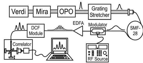
Fig. 3. Experimental setup for realization of subpicosecond pulse shaping. OPO, optical parametric oscillator.
