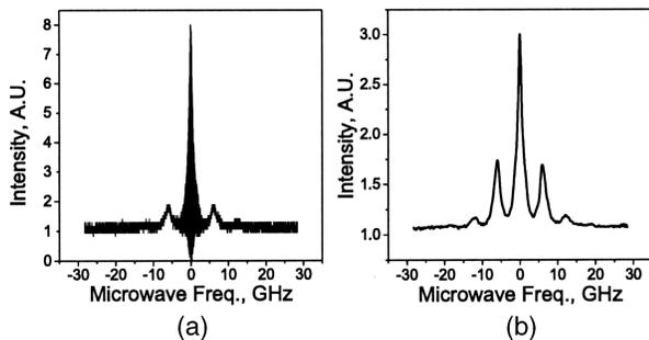
Fig. 3. (a) Interferometric correlation for 6-GHz modulation. (b) Intensity correlation.
