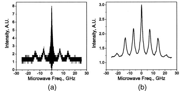
Fig. 2. (a) Interferometric correlation, showing microwave signal at  $f_m = 7 \text{ GHz}$ . (b) Intensity correlation reveals the enhancement of second and third harmonics from nonlinear modulation.
