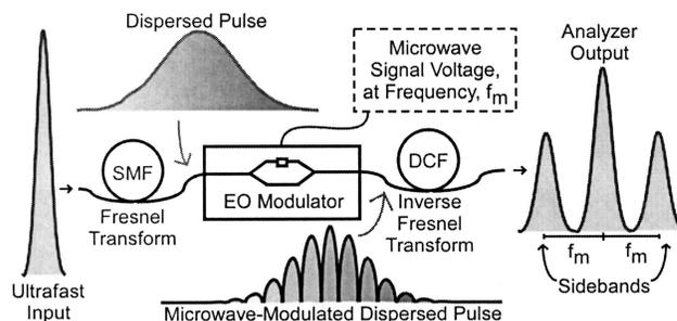
Fig. 1. General microwave analyzer approach to microwave spectrum analysis by use of dispersive fiber for signal processing.
