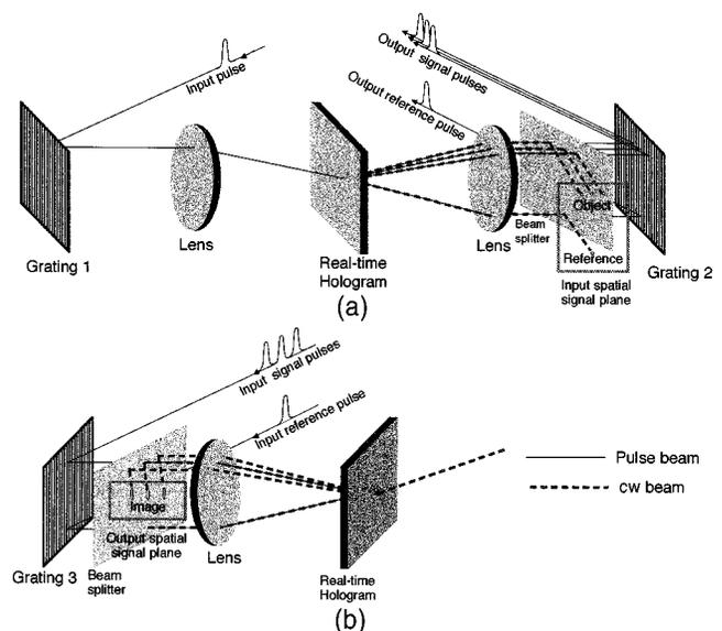
Fig. 1. Schematic diagram of optical processors for (a) parallel-to-serial and (b) serial-to-parallel conversions.
