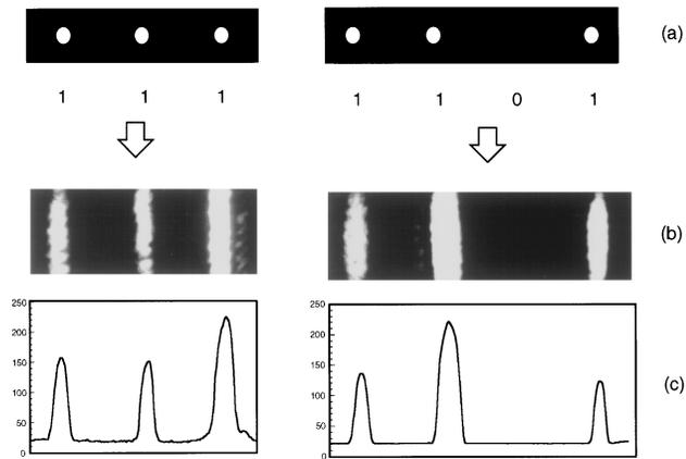
Fig. 3. Experimental results of image transmission with parallel-to-serial and serial-to-parallel conversion: (a) photograph of the 1-D input data arrays, (b) photograph of the 1-D binary data array images reconstructed at the receiver, (c) plots of the intensity distributions in (b).
