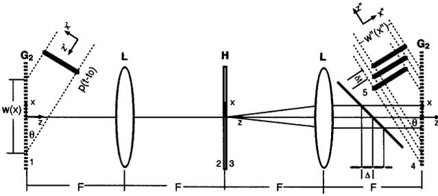
Fig. 2. Schematic diagram of parallel-to-serial conversion with four-wave mixing in real-time holograms: L's, lenses; H, hologram.
