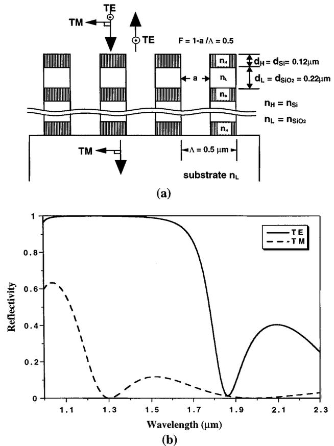
Fig. 1. (a) Schematic diagram of an ASR PBS operated with plane waves at normal incidence. (b) Numerical results of the reflectivity for TE- and TM-polarized waves versus wavelength of a seven-layer PBS designed for normally incident waves.
