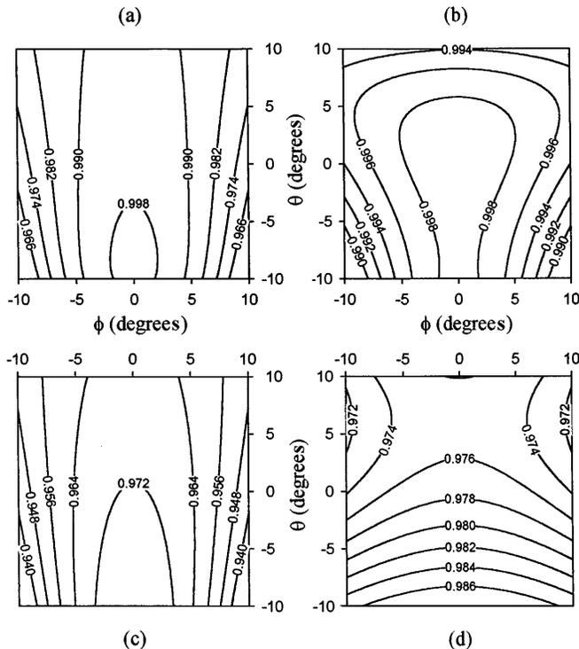
Fig. 3. Contour plots of TE reflectance and TM transmittance versus incident angles  $(\phi, \theta)$  as defined in Fig. 2(a): (a) TE reflectance at wavelength  $\lambda = 1.3 \mu\text{m}$ , (b) TM transmittance at wavelength  $\lambda = 1.3 \mu\text{m}$ , (c) TE reflectance at wavelength  $\lambda = 1.5 \mu\text{m}$ , and (d) TM transmittance at wavelength  $\lambda = 1.5 \mu\text{m}$ .
