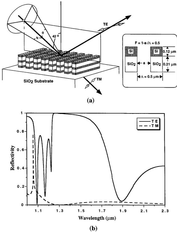
Fig. 2. (a) Schematic diagram of five-layer ASR PBS operated with incident waves at an angle of  $42^\circ$ . (b) Numerical results for the reflectivity of TE- and TM-polarized waves versus wavelength for  $42^\circ$  incidence.
