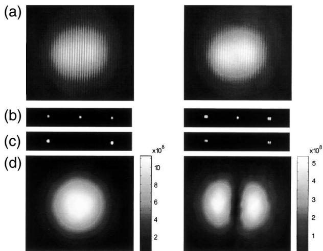
Fig. 3. (a) Interference patterns, observed for two relative time delays, separated by  $\Delta\tau \sim 6$  ps. Two-dimensional spatial Fourier spectrum (b) before and (c) after filtering, showing dc and ac terms in each case in the center and on the sides, respectively. (d) Reconstructed modal intensity distributions corresponding to left,  $LP_{01}$  and right,  $LP_{11}$  modes.
