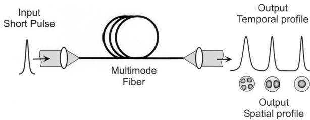
Fig. 1. Propagation of an optical pulse in a multimode fiber. A single input pulse excites a set of spatial propagation modes of the fiber, which appear at the output at different times.
