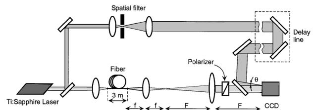
Fig. 2. Experimental setup for interferometric cross-correlation measurements.
