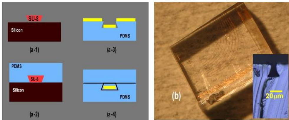
Figure 6. (a) Soft lithography method for creating gold patterns embedded in PDMS. (b) A PDMS sample with 8 micron wide metal wires embedded in it. Inset shows a cross section of PDMS after it was removed from the mold.
