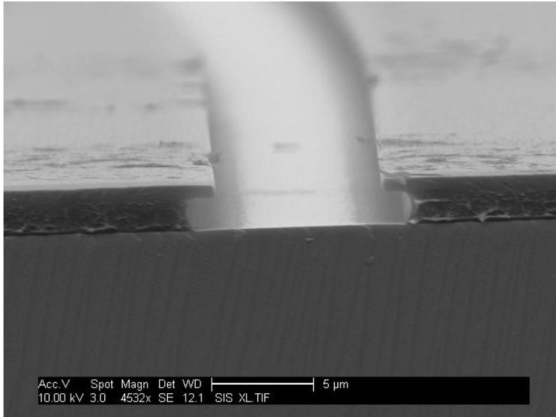
Figure 2. Controllable photoresist undercut using PMGI for metal liftoff. Photoresist is Shipley S1805.
