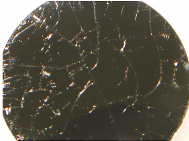
Figure 4. Cracks in S1805 photoresist on a PDMS substrate, spun on top of a silicon wafer.
