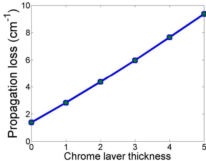
Figure 3. The detrimental effect of a chrome adhesion layer simulated using a finite element mode solver (COMSOL Multiphysics).
