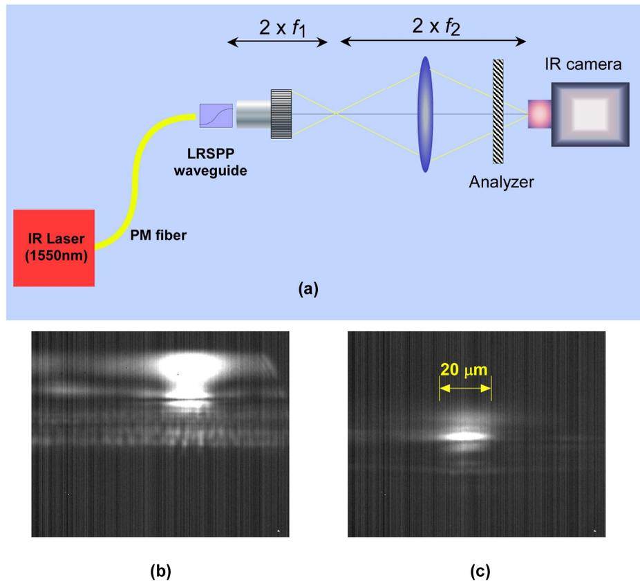
Figure 7. (a) Optical setup for characterizing the LRSPP waveguides. (b) Output of SU-8 clad waveguide when a dielectric slab mode is excited(c) Output of SU-8 clad waveguide with correct end-fire excitation. The mode is a TM mode.
