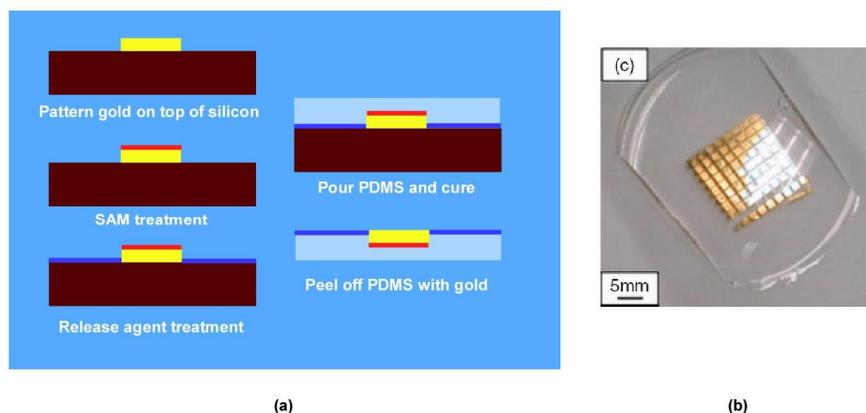
Figure 5. Method of gold pattern transfer to PDMS using self assembled monolayers (SAMs). (from Lee *et al.* [Ref]) .
