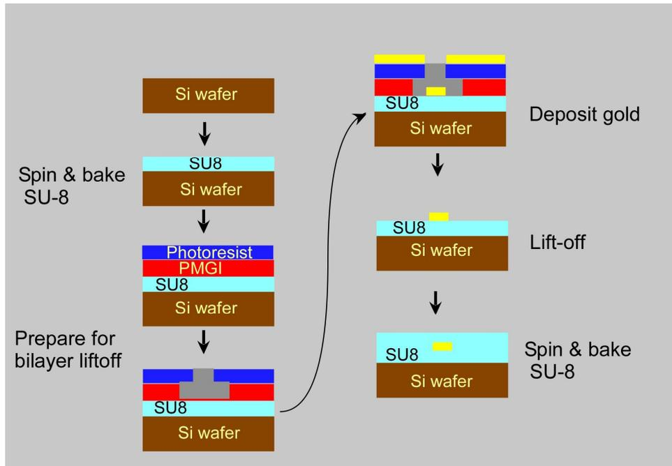
Figure 1. Fabrication steps for creating metal stripe waveguides in SU-8.
