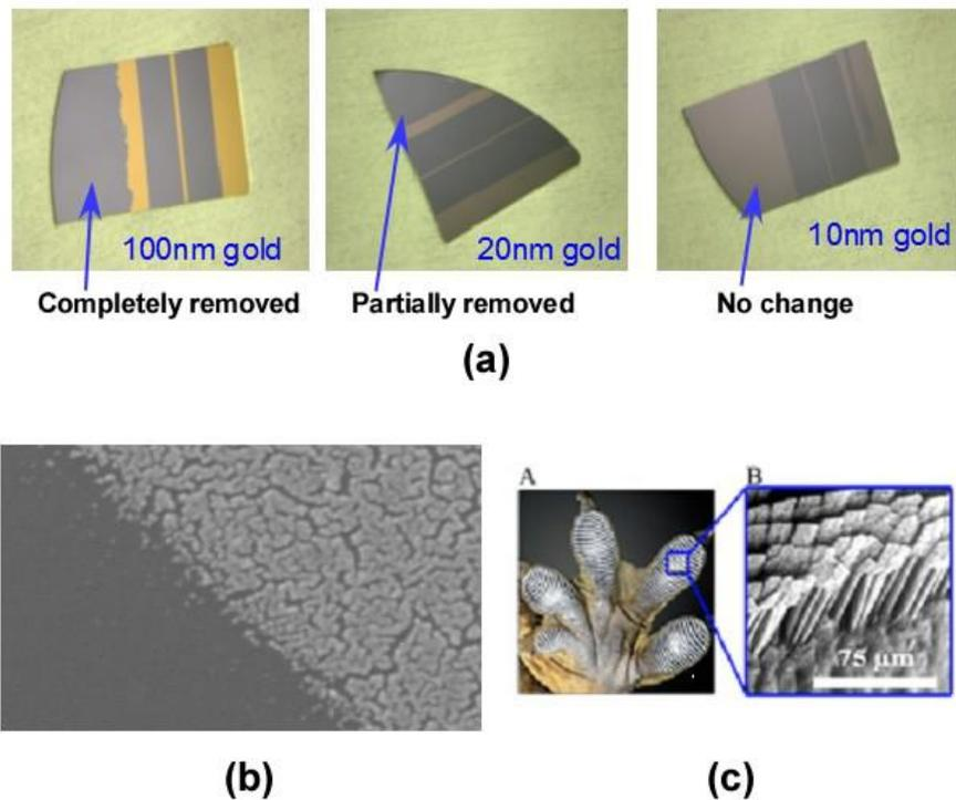
Figure 8. Results of gold adhesion experiment. (a) Different samples showing the success of gold film removal using tape (b) SEM of a nominally 10nm thick gold film. (c) Image of a gecko's foot, showing the microstructured array of setae, which enable it to climb walls.
