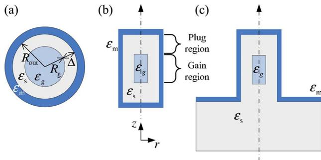
Fig. 1. (Color online) (a) Cross section of the metal-coated composite gain waveguide. (b) Cylindrical closed 3D resonator. (c) Cylindrical open 3D resonator.
