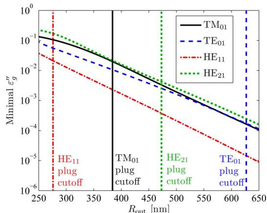
Fig. 3. (Color online) Minimal threshold gain as a function of  $R_{\text{out}}$ . The vertical lines show the cutoff of each mode in the 3D resonator plug region.
