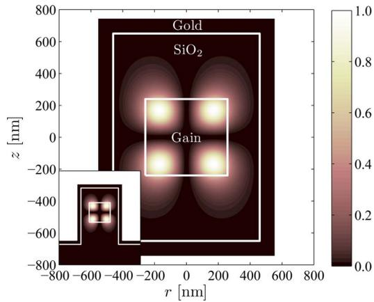
Fig. 4. (Color online) Cross section of a closed cylindrical 3D subwavelength laser resonator. The electric field intensity  $|\vec{E}|^2$  normalized to its maximal value of the  $TE_{012}$  mode is shown. The inset shows a similar open structure.
