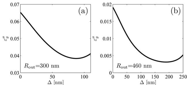
Fig. 2. Threshold gain  $\varepsilon_g''$  as a function of the shield thickness  $\Delta$  for the  $\text{TE}_{01}$  mode. (a)  $R_{\text{out}}=300$  nm. (b)  $R_{\text{out}}=460$  nm.
