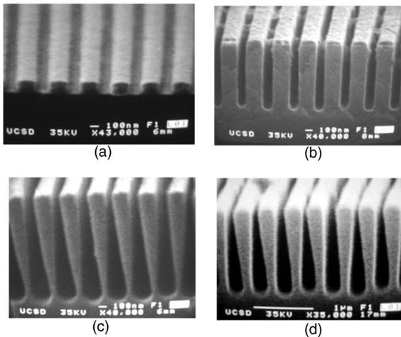
**Fig. 1** SEM micrographs of 400-nm-period grating transferred to a GaAs substrate using CAIBE: (a) SU-8 resist mask with 150-nm thickness; (b) structure of 980-nm depth etched using 20-sccm  $\text{Cl}_2$  flow; (c) 1480-nm depth using 18 sccm  $\text{Cl}_2$  flow; (d) 1440-nm depth using 14-sccm  $\text{Cl}_2$  flow.
