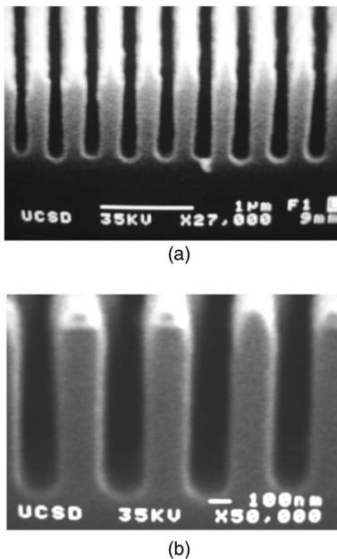
**Fig. 2** SEM micrographs of GaAs grating structure with period of 400 nm etched in CAIBE using SU-8 resist layer as mask: (a) overetched structure using 7-sccm  $\text{Cl}_2$  flow; (c) smooth vertical etched structure with 790-nm depth using 6-sccm  $\text{Cl}_2$  flow.
