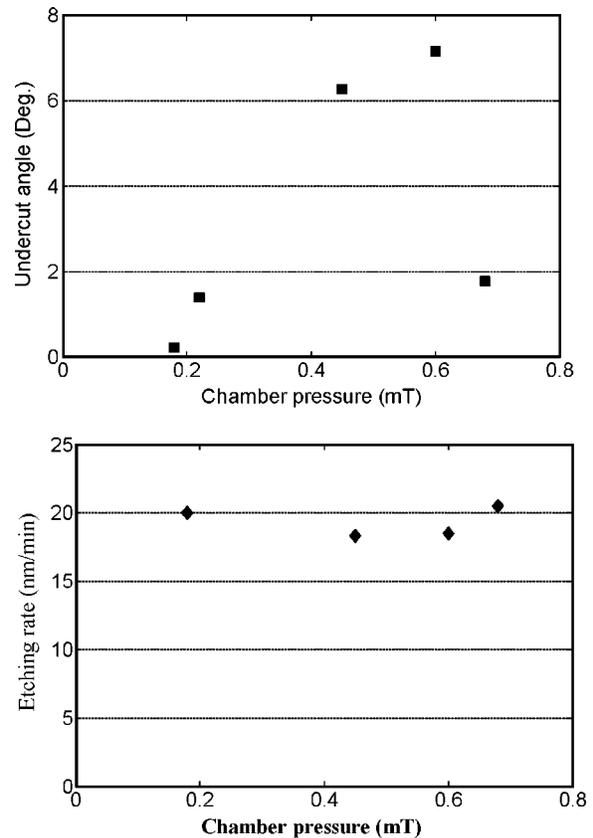
**Fig. 3** Dependence of (a) the undercut angle of the etched profile and (b) the etching rate of GaAs on the chamber pressures.
