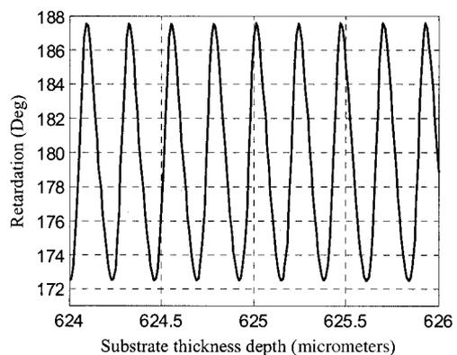
Fig. 5. Variation in retardation versus the substrate thickness with no antireflection coating on the back side for a grating depth of 880 nm and duty cycle of 0.70.
