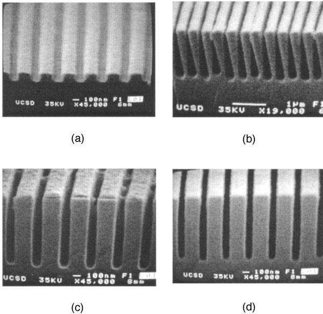
Fig. 3. SEM photographs of submicrometer gratings: (a) SU-8 mask with a 350-nm period and aspect ratio of 0.6, (b) transferred structure in GaAs with an inverse taper profile by use of the thin-layer SU-8 (a) as the dry-etching mask, (c) improved but contaminated profile, (d) smooth and vertical sidewall structure in GaAs with an aspect ratio of 4 and thickness of 950 nm.
