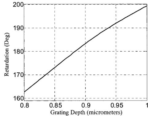
Fig. 4. RCWA-generated curve showing the effect of etch depth on the total retardation of a grating etched in GaAs at 1550 nm ( $n = 3.37$ ). The nominal duty cycle and grating period are assumed to be 0.70 and 325 nm, respectively. Half-wave retardation is obtained for a grating depth of 880 nm.
