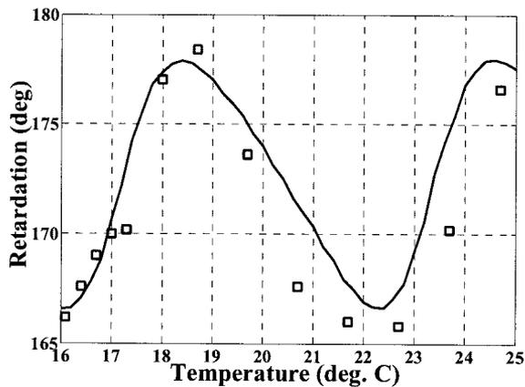
Fig. 6. Variation in retardation of the fabricated sample versus temperature (rectangular markers) and fitted theoretical curve obtained with RCWA. The fitted grating is having a duty cycle, period, and etch depth equal to 0.71, 325 nm, and 850 nm, respectively.
