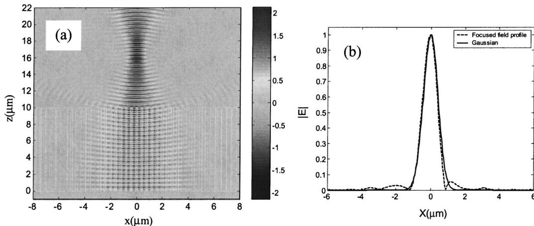
Fig. 6. Field propagation through a focusing graded-index lens with  $n_0 = 3$ ,  $\alpha = 0.01$  ( $1/\mu\text{m}^2$ ). The initial beam diameter is  $6.5 \mu\text{m}$ . (a) Top view showing the focusing effect. (b) Cross section at the focus. For comparison purposes, the Gaussian beam profile is also displayed.
