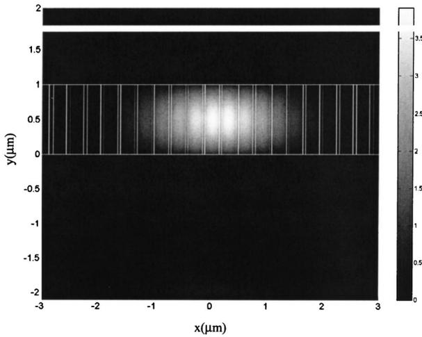
Fig. 4. Typical beam cross section traveling along subwavelength-based graded-index media. The structure is composed of a  $1\text{-}\mu\text{m}$  GaAs slab layer on top of an aluminum oxide cladding layer. The GaAs layer is patterned with a structure having a period of  $\Lambda = 0.3 \mu\text{m}$ . The duty ratio is calculated according to Eq. (1a) to achieve an effective index profile with  $n_0 = 3.1$  and  $\alpha = 0.01 (1/\mu\text{m}^2)$ .
