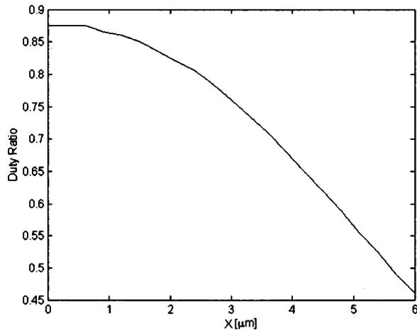
Fig. 2. Duty ratio versus lateral distance from the optical axis for TE polarization:  $n_0 = 3.2$ ,  $\alpha = 0.01$  ( $1/\mu\text{m}^2$ ),  $\lambda = 1.55$   $\mu\text{m}$ ,  $\Lambda = 0.3$   $\mu\text{m}$ ,  $n_1 = 3.37$ ,  $n_2 = 1$ .
