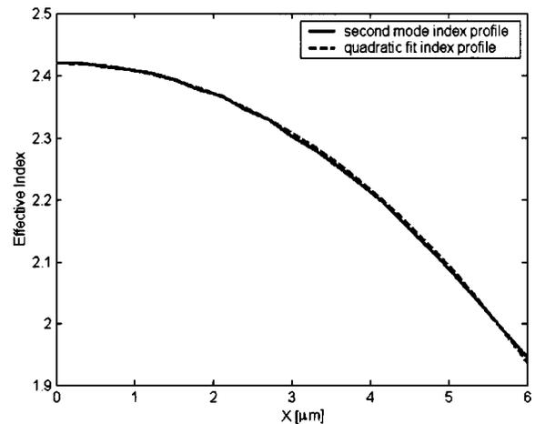
Fig. 5. Effective index of the second slab mode for a quadratic profile optimized for the first mode. Solid curve, obtained index profile; dashed curve, fitting to a modified quadratic profile with  $n'_0 = 2.42$ ,  $\alpha' = 0.01 (1/\mu\text{m}^2)$ . Slab thickness is  $0.65 \mu\text{m}$ , with an effective index of 3.19 and 2.61 for the two modes, respectively.
