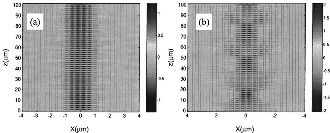
Fig. 8. Field propagation through a subwavelength-based graded-index waveguide with the effective index parameters  $n_0 = 3$ ,  $\alpha = 0.01$  ( $1/\mu\text{m}^2$ ). The beam diameter at the front end of the structure was chosen to be (a)  $2.4 \mu\text{m}$ , (b)  $4.5 \mu\text{m}$ . In (a) a supercollimation characteristic is demonstrated since the diffraction and the focusing power are balanced.
