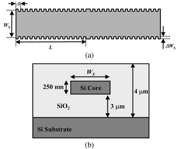
Fig. 1. (a) Schematic diagram of the top view of quarter wavelength shifted transmission resonant filter with vertical gratings, where  $W_S$  is the average width of the waveguide,  $\Delta W_S$  is the full depth of a single side of the vertical grating, and  $L$  and  $\Lambda$  are the total length and the period of a single Bragg reflector, respectively. (b) Cross section of the transmission resonant filter.
