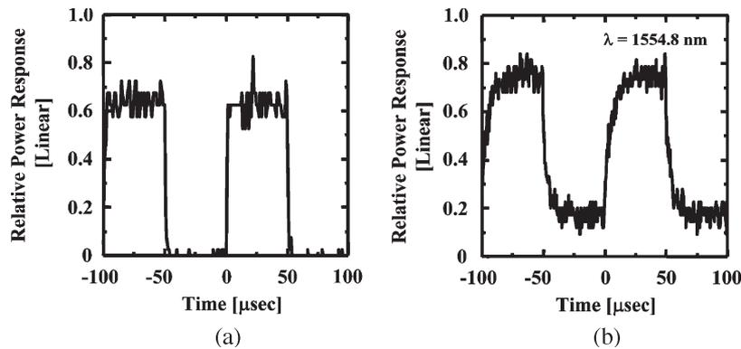
Fig. 6. (a) Power versus time trace of the modulated argon laser beam used to pump the cavity region of the device. (b) Output power versus time of the device operating at a wavelength of  $\lambda = 1554.8$  nm, when the cavity region of the device is modulated by the modulated argon laser with an average power of about 1.5 mW.
