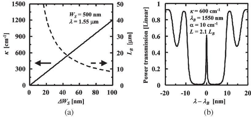
Fig. 2. (a) Calculated coupling coefficient ( $\kappa$ ) and corresponding Bragg length ( $L_B = 1/\kappa$ ) versus  $\Delta W_S$ . (b) Simulated transmission power versus  $(\lambda - \lambda_B)$ .
