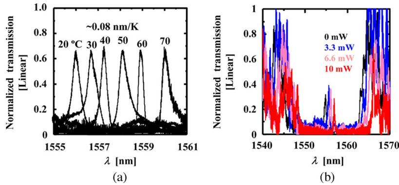
Fig. 5. (a) Transmission spectra of the resonant mode for substrate temperature varying in the range of 20 °C–70 °C. (b) Transmission spectra of the resonant mode for irradiance of the cavity region of the device by the CW argon laser at power levels varying in the range of 0–10 mW.
