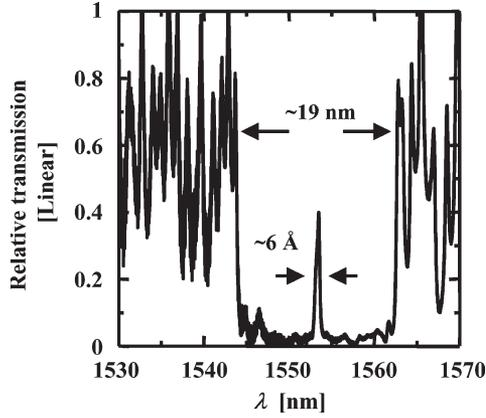
Fig. 4. Measured transmission spectrum of the device at TE polarization.
