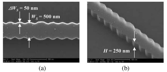
Fig. 3. Scanning electron micrographs of a dry etched device sample. (a) Top view. (b) Tilted view.
