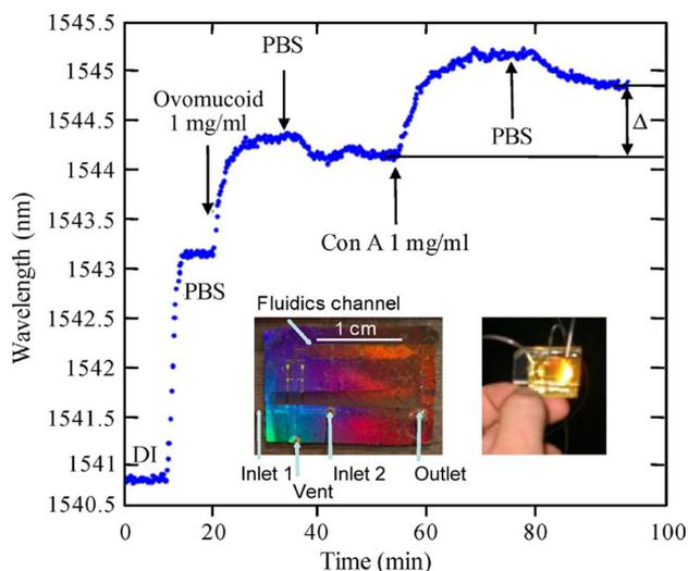
Fig. 3. Demonstration of protein-carbohydrate binding on a gold nanohole array observed by monitoring the resonant wavelength of a SPP mode at the fluid-metal overlayer in a transmission setup. Insets are photographs of an SPP sample holder with (right) and without (left) tubing.
