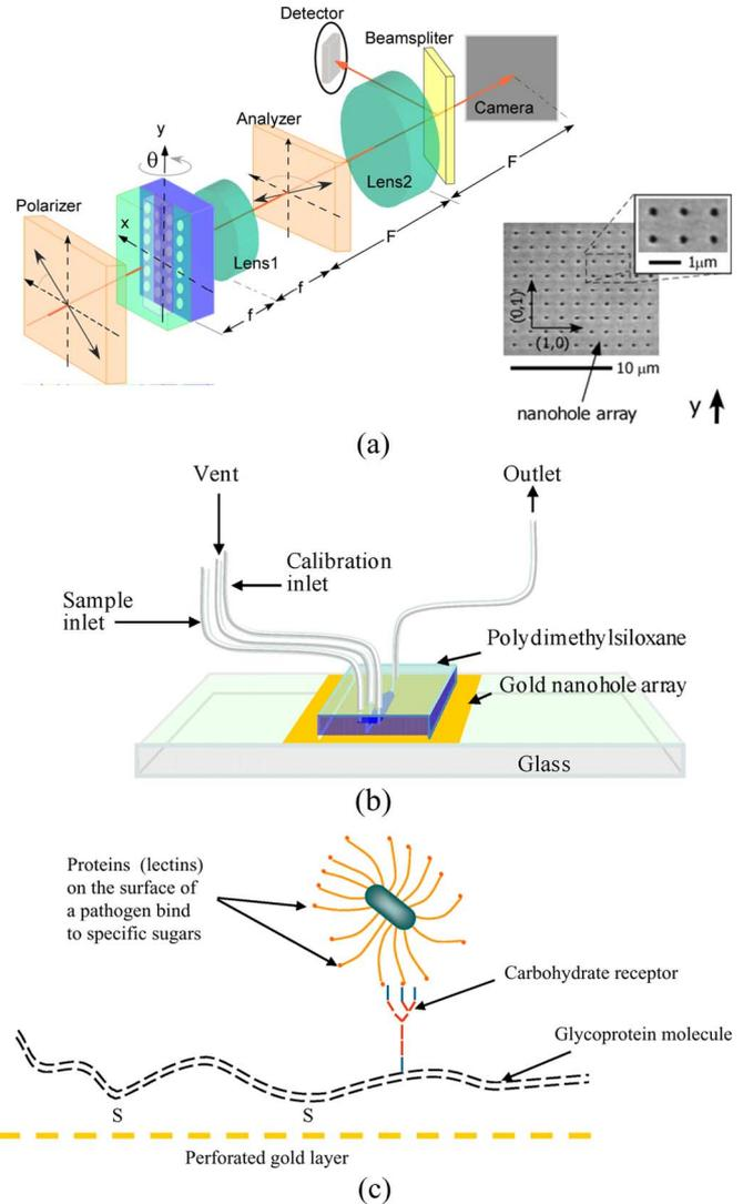
Fig. 1. (a) Schematic of the 2-D nanohole-array SPP transmission setup. Inset: scanning electron micrograph of a section of the gold nanohole array. (b) SPP sample holder. (c) Pathogen capture via carbohydrate receptor and protein binding.
