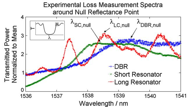
**Fig. 4** Transmission spectra of the experimental structures about the null reflectance point. The *inset* in the *upper left* of the figure is a conceptual illustration in which the *shaded area* indicates the approximate position of the measurements relative to the DBR stopband
