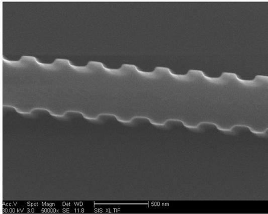
**Fig. 2** Scanning electron micrograph of an uncladded section of DBR. Note that the *scale bar* label is 500 nm
