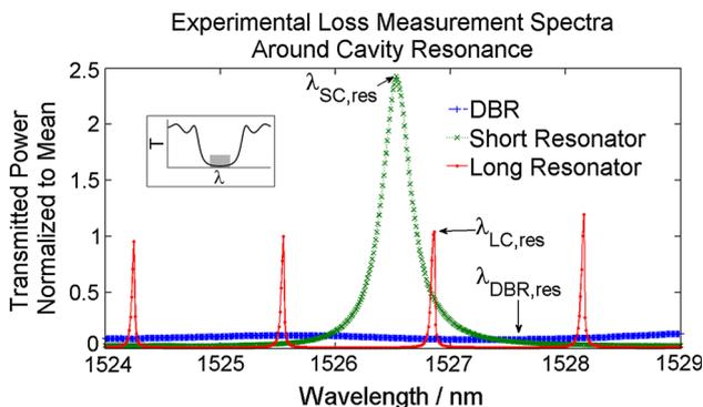
**Fig. 3** Transmission spectra of the experimental structures about the cavity resonance. The *inset* in the *upper left* of the figure is a conceptual illustration in which the *shaded area* indicates the approximate position of the measurements relative to the DBR stopband
