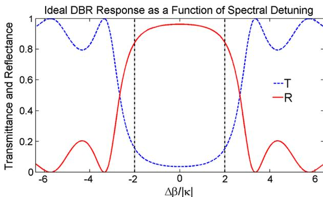
**Fig. 1** Dependence of the response of an ideal DBR on spectral detuning. In this example,  $|\kappa| = 600 \text{ cm}^{-1}$  and  $L_{\text{DBR}} = 38.912 \text{ }\mu\text{m}$ . Vertical lines denote the conventional edge of the stopband
