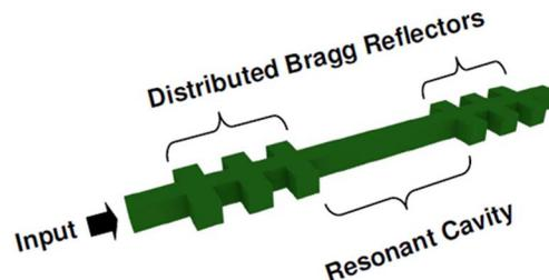
Fig. 1. Top-down diagram of a Fabry–Pérot resonator created from a pair of distributed Bragg reflectors in a strip waveguide. Note that the diagram is for conceptual purposes and is not drawn to scale.
