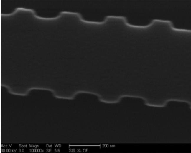
Fig. 2. Scanning electron micrograph of an uncladded section of the SOI strip waveguide distributed Bragg reflector employed in this experiment. Note that the scale bar label is 200 nm.
