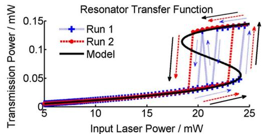
Fig. 6. Measurements and theoretical response of the transfer function of the quasi-TE mode of the distributed Bragg reflector Fabry–Pérot resonator. Run 1 and Run 2 were made 8 min apart. Point-by-point measurements are taken at an average rate of  $0.77 \text{ Hz}$ . The wavelength detuning from resonance of the model is  $0.15 \text{ nm}$ .
