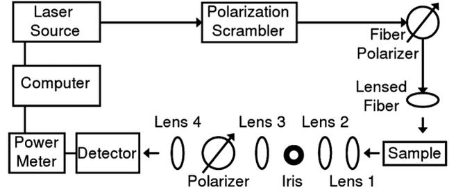
Fig. 3. Experimental setup used to characterize the device. The details of the components used may be found in the text.
