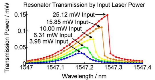
Fig. 5. Power dependence of the transmission around the 1547 nm resonance peak of the quasi-TE mode of the distributed Bragg reflector Fabry-Pérot resonator.
