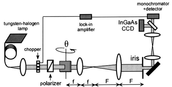
Fig. 4. Apparatus for optical characterization. The broadband incident beam is collimated and polarized. The sample is then  $4f$  imaged via a lens onto a pinhole for alignment and control of the measurement area and  $4f$  imaged again onto an InGaAs CCD and spectrum analysis setup.
