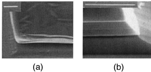
Fig. 3. (a) Scanning-electron microscope image of the fabricated mesa structure and subsequent delamination. (b) Mesa structure intact after *in situ* annealing as described in the text. Scale for bars in both images, 10  $\mu\text{m}$ .
