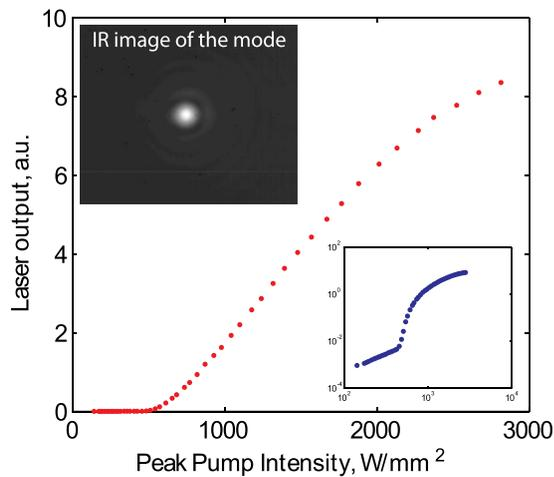
FIG. 4. The laser light-light curve in linear and logarithmic (lower right inset) scale with the IR image (upper left inset) of the lasing mode; lasing threshold is at  $530 \text{ W/mm}^2$ .
