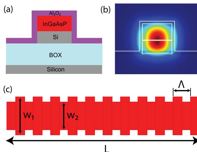
FIG. 1. III-V/Si hybrid DFB laser design: schematic drawing of a III-V/Si DFB laser resonator with vertical sidewall modulated Bragg gratings—cross-section (a) and top view (c); (b) finite element simulation (COMSOL) of a fundamental TE-like mode for a 500 nm wide and 550 nm tall III-V/Si waveguide with 250 nm silicon layer, 300 nm InGaAsP MQW layer, and 50 nm  $\text{Al}_2\text{O}_3$  cladding.
