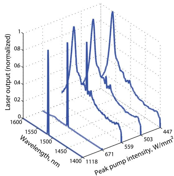
FIG. 3. Spectral evolution, with final peak wavelength at 1515 nm.
