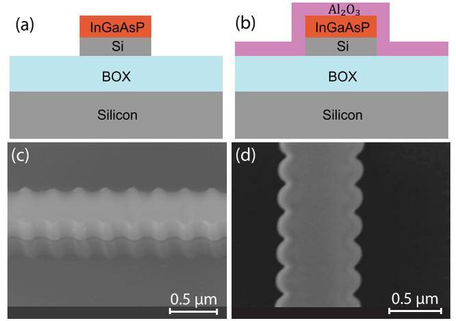
FIG. 2. (a), (b) Schematic steps of fabrication process; (c), (d) the SEM images of the Bragg grating after two-step RIE and after  $\text{Al}_2\text{O}_3$  layer deposition by ALD, respectively.
