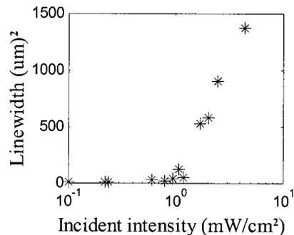
Fig. 6. Dependence of width of the scanned line in SU-8 on incident intensity by a 36 $\times$  reflective MO with the square of the linewidth as a function of the intensity on logarithmic scale.
