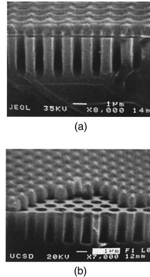
Fig. 5. SEM micrograph of 2-D photonic crystals with period of 1.5  $\mu\text{m}$  transferred into a GaAs substrate by CAIBE: (a) orthogonal lattice with a 3- $\mu\text{m}$  depth in a GaAs substrate; (b) a hexagonal periodic structure with a 3- $\mu\text{m}$  depth.
