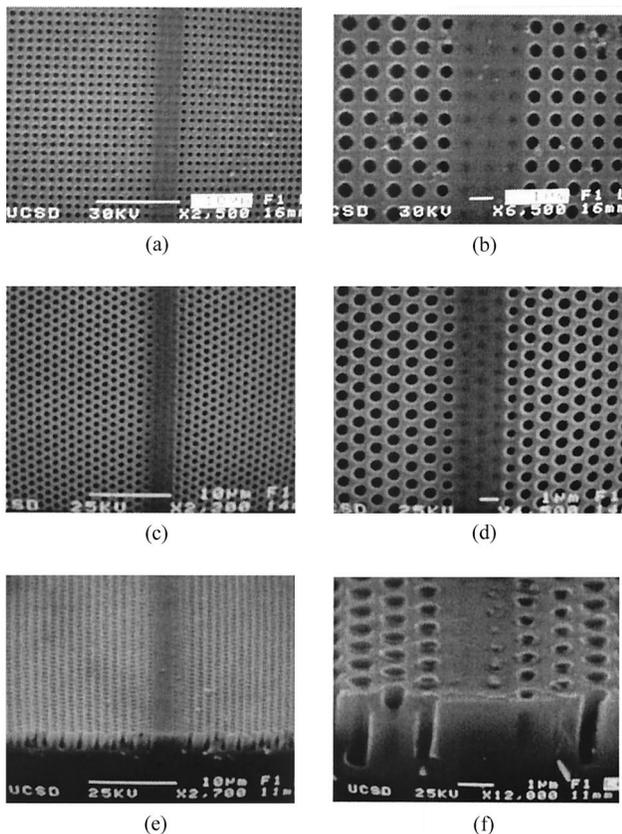
Fig. 7. SEM photographs of (a) a line defect introduced into a rectangular mesh photonic crystal lattice in SU-8; (b) a magnified view of (a) demonstrating the possibility of large-area fabrication with good quality; (c) a line defect introduced into a hexagonal lattice structure with three lines of holes canceled; (d) a magnified view of (c); (e) a line defect transferred into the GaAs substrate with two lines of the hole canceled; (f) a magnified view of (e).
