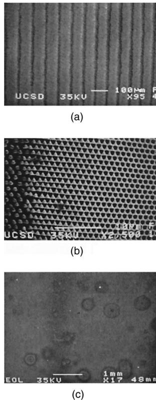
Fig. 4. SEM photographs of a hexagonal lattice structure in SU-8 to show the beat period that is due to the misalignment of the substrate rotations: (a) result from use of a manually controlled rotation stage; (b) magnified transition areas in (a); (c) result obtained with a high-precision Physik Instrumente rotating stage with perfect hole areas approximately 2 mm wide.
